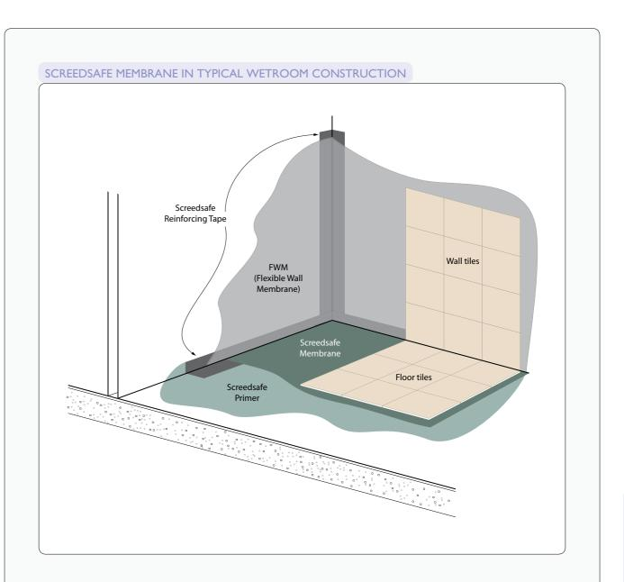
For solid floors we recommend that the Screedsafe membrane is applied to the shower area plus an additional one metre in either direction.
