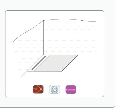
Consisting of three main elements, the Modular Wet-Floor is simple to configure. Start by selecting the required number of Drainage Components and Tapered Boards, then simply choose the appropriate Floor or Wall Grill to suit your wetroom layout.
