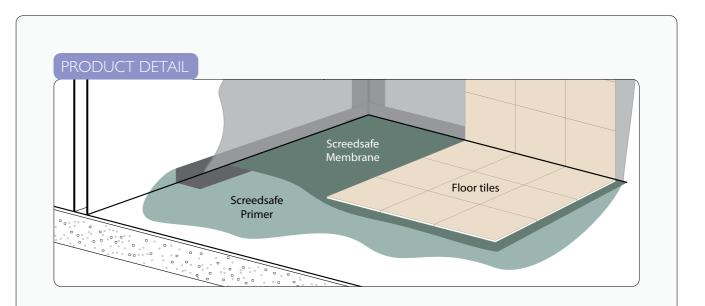
Screedsafe is a self-adhesive waterproof membrane designed for use prior to the application of ceramic tiles, and natural stone onto concrete and screeded in wetrooms and other critical areas.
