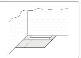
For layout 5 we recommend a maximum width of 1700mm, for widths greater than this use two Drainage Components, as layout 7.
