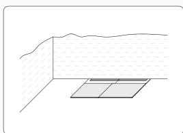
For layout 8 the minimum width required is 1800mm
