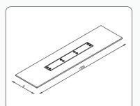
\*When installed with the Wall Grill, the Drainage Component width is reduced by 80mm, to 220mm.
